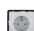
2P+PE with OP schuko outlet single, with safety shutters and overvoltage protection (LIGHT INDICATION) 16 A, 250 V AC
