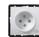
2P+PE with OP outlet single, with safety shutters and overvoltage protection (AUDIBLE ALARM) 16 A, 250 V AC
